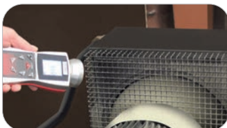
Stroboscope off: rotations not visible
