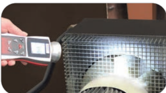
Stroboscope on: rotations visible
