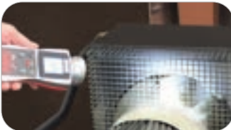
Stroboscope on: rotations visible
