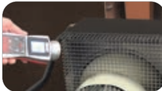
Stroboscope off: rotations not visible
